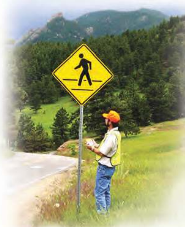
Boulder County, Colorado's Road Maintenance Department uses ArcPad to map out thousands of road signs and collect attribute information including type, condition, and location.
