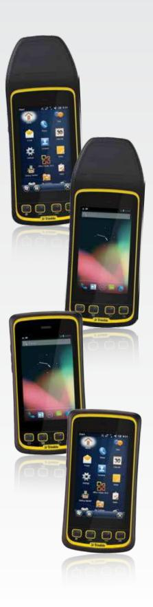
The flexible, fully rugged Juno T41 is available in a wide variety of configurations. Build the handheld computer you need: Android or Microsoft Windows operating systems, Barcode Imager, Smartphone or GPS collector (or both)... whatever your ideal combination of features and functionality, the Juno T41 is a reliable workhorse designed to last for years in any environment.
