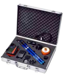
Above image shows the Vertex Laser Geo 360 system with charger and cable, in transport case.
