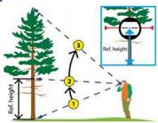
Stand at a distance approximately as far away from the object and the object's height for best results. The reference height mark should be set at 2 meters/6feet.
